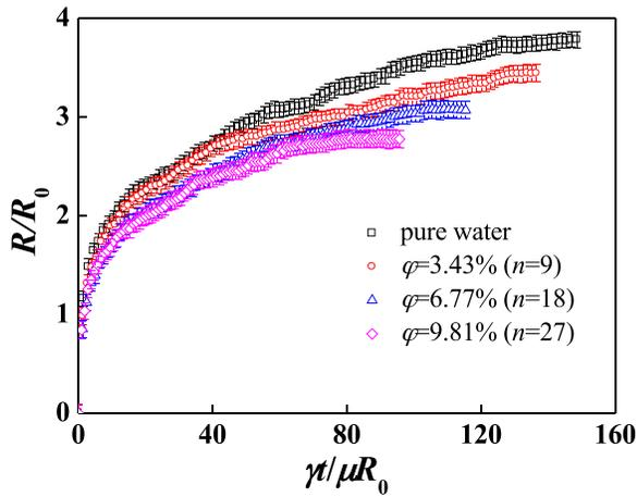
FIG. 2. Dimensionless spreading radius as a function of the dimensionless time for cylindrical water nanofluid droplets containing Au nanoparticles of volume fractions of 0%, 3.43%, 6.77%, and 9.81% on a Au(100) substrate. Error bars are obtained by using four different random velocity seeds for temperature initializations.
