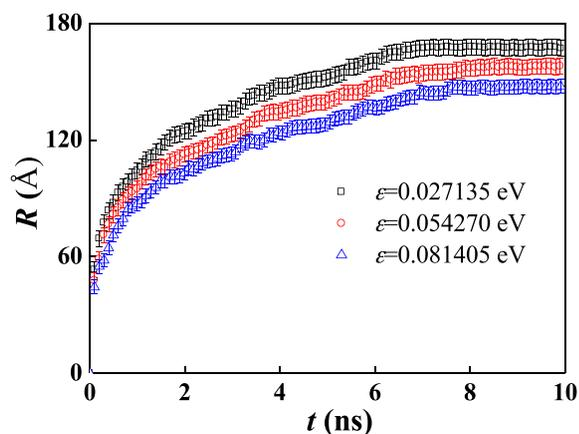
FIG. 4. The spreading radius as a function of spreading time for nanofluid droplets with different particle wettabilities for particle volume fraction of  $\varphi = 9.81\%$ . Error bars are obtained by using four different random velocity seeds for temperature initializations.
