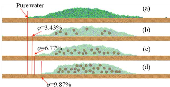
FIG. 1. Snapshots of nanoscale water droplet containing Au nanoparticles of various volume fractions spreading on a Au(100) surface of 300 K at  $t=10$  ns: (a) pure water; (b) nanofluid of  $\phi=3.43\%$  ( $n=9$ ); (c)  $\phi=6.77\%$  ( $n=18$ ); (d)  $\phi=9.81\%$  ( $n=27$ ). Water molecules are made semi-transparent for a better visualization of nanoparticles within the droplets from (b)–(d).
