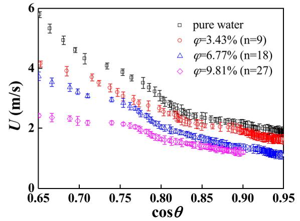
FIG. 3. The contact line velocity,  $U$ , as a function of  $\cos \theta$  ( $\theta$  is the dynamic contact angle) for water-gold nanofluid droplets with particle volume fractions of 0%, 3.43%, 6.77%, and 9.81%. Error bars are obtained by using 4 different random velocity seeds for temperature initializations.
