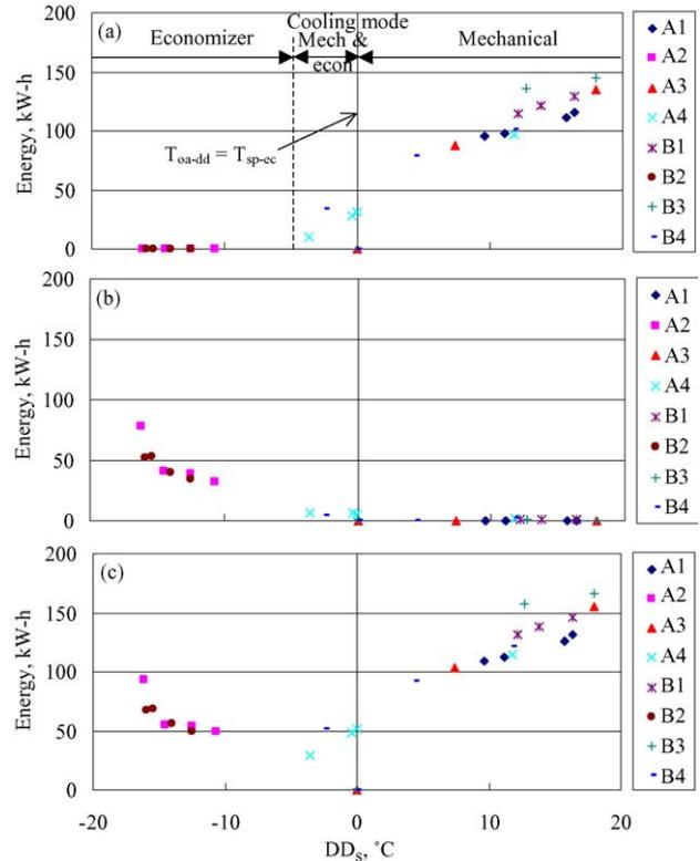
Fig. 10. Energies for hydronic reheat. (a) Cooling coil; (b) Hydronic reheat; (c) Total energy.
