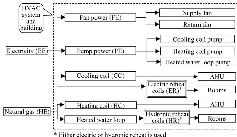
Fig. 6. Schematic diagram of electricity and natural gas energy usage.
