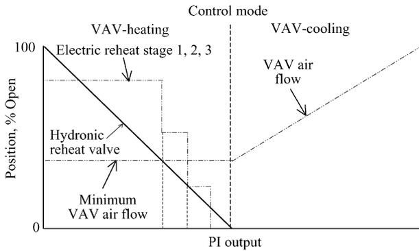
Fig. 5. Room temperature control sequence.
