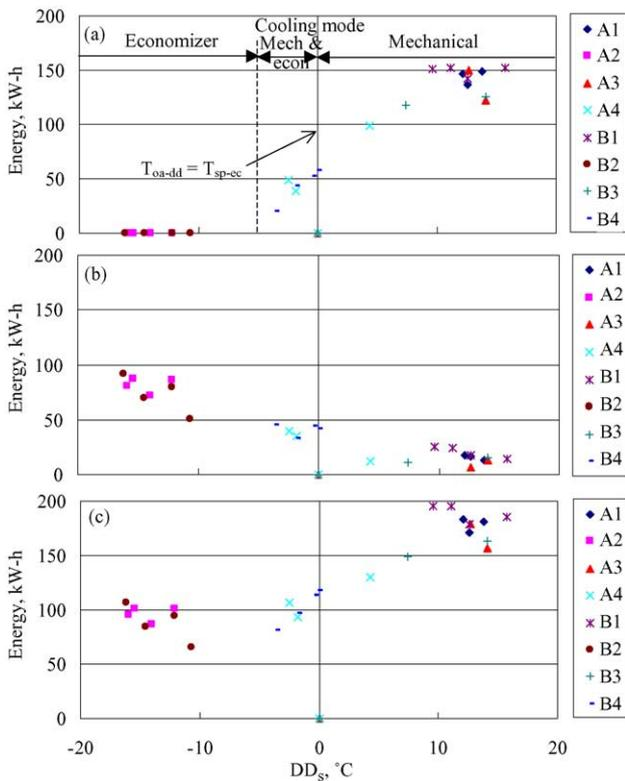
Fig. 9. Energies for electric reheat. (a) Cooling coil; (b) Electric reheat; (c) Total energy.
