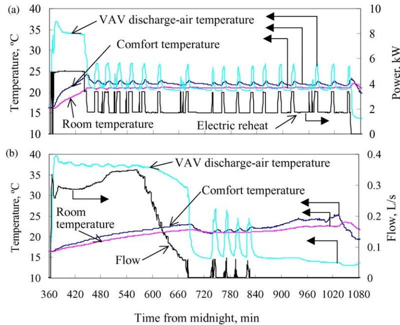
Fig. 8. Economizer cooling mode for West B-Room. (a) Power and temperatures for electronic reheat (13 March 2001); (b) Water flow and temperatures for hydronic reheat (3 March 2001).
