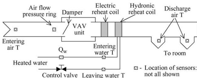
Fig. 3. VAV with reheat unit and associated equipment [11].
