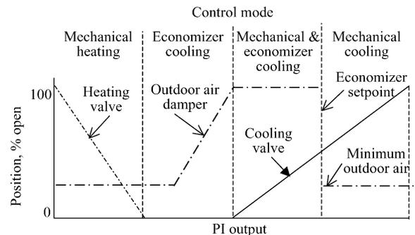
Fig. 4. Supply air temperature control sequence [11].
