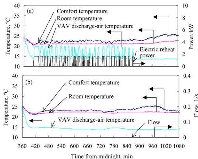
Fig. 7. Mechanical cooling mode for West B-Room. (a) Power and temperatures for electric reheat (12 July 2000); (b) Water flow and temperatures for hydronic reheat (2 July 2000).
