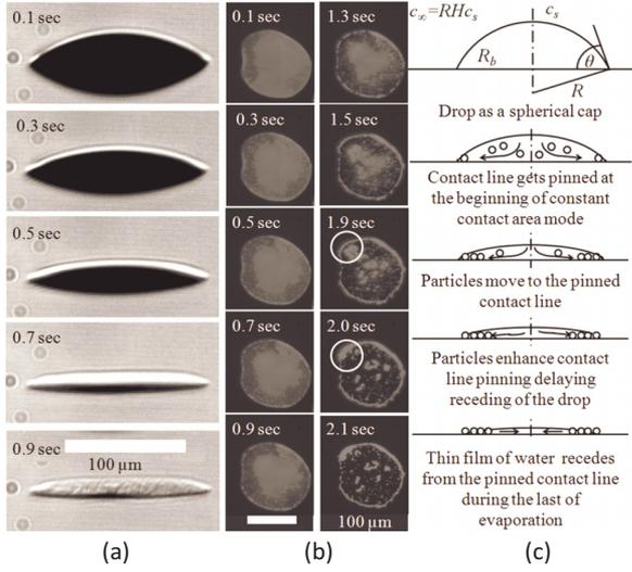
FIG. 1. (Color online) Snapshots of a drying colloidal drop at 60% relative humidity on a glass substrate from (a) side view, (b) bottom view, and (c) schematic of the pinned evaporation process. Particle movement toward the pinned contact line can be observed clearly between 1.9 and 2 s (circled areas).
