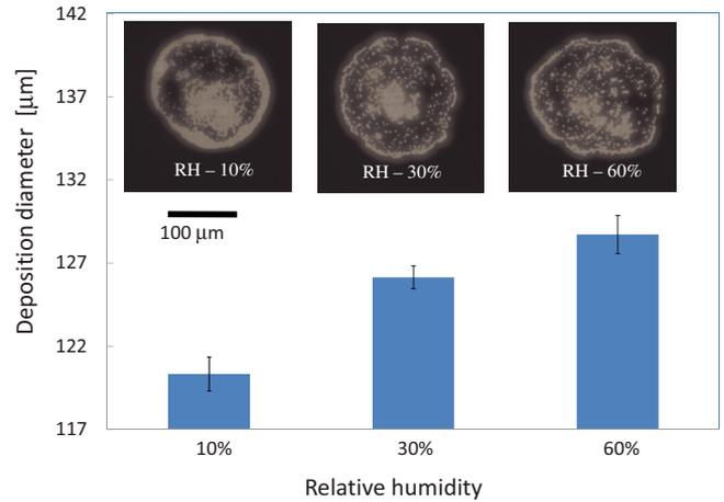
FIG. 3. (Color online) Final deposition morphology as a function of the RH. The scale bar (100  $\mu\text{m}$ ) is the same for all images.
