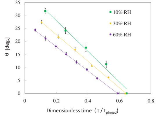
FIG. 2. (Color online) Contact angle of the drop as a function of nondimensional time at different RH values.
