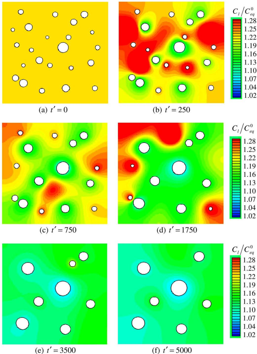
**Fig. 9.** Simulation of coarsening of hydrogen bubbles in an aluminum melt without flow. The black lines are the  $\phi = 0.5$  phase-field contour and the colors indicate the hydrogen concentration in the liquid. The initial gas volume fraction is 5.5%. (For interpretation of the references to color in this figure legend, the reader is referred to the web version of this paper.)
