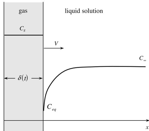
Fig. 1. Growth of a gas layer in a supersaturated liquid.
