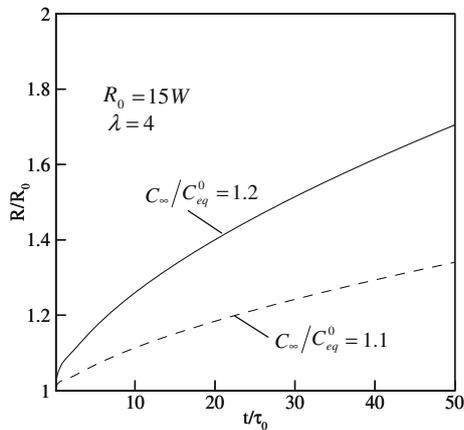
Fig. 6. Predicted evolution of the dimensionless radius of a hydrogen bubble growing into an infinite, supersaturated aluminum melt.
