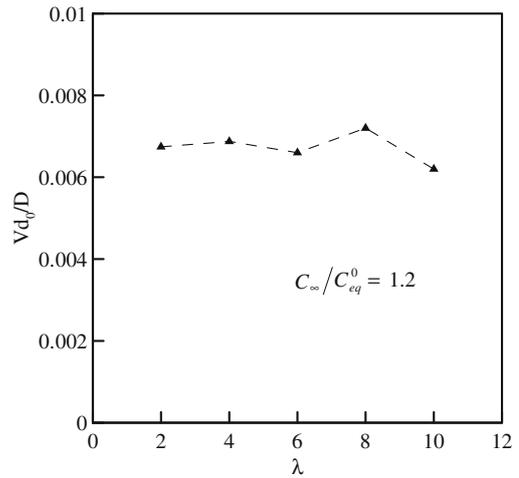
Fig. 8. Convergence of the predicted gas-liquid interface velocity with respect to the diffuse interface coupling constant  $\lambda$  for growth of a hydrogen bubble in a supersaturated aluminum melt ( $Dt/d_0^2 = 5134$ ).
