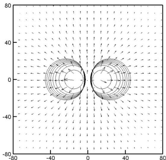
**Fig. 12.** Simulation of the growth of two equal-sized hydrogen bubbles in an isothermal, supersaturated aluminum melt with flow in the liquid and inside the bubbles. The predicted interface contours are shown every 2000 time steps, while the velocity vectors are for the last time step only.
