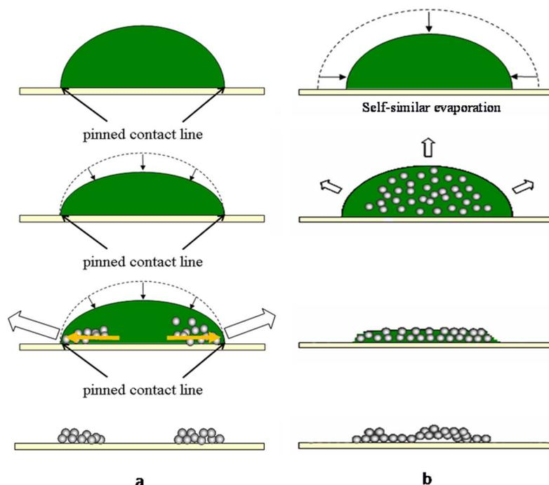
Fig. 1. Colloidal drop deposition for different evaporation mechanisms. (a) Pinned contact line leading to coffee ring deposits. (b) Constant contact angle and mixed mode leading to relatively more uniform deposits.
