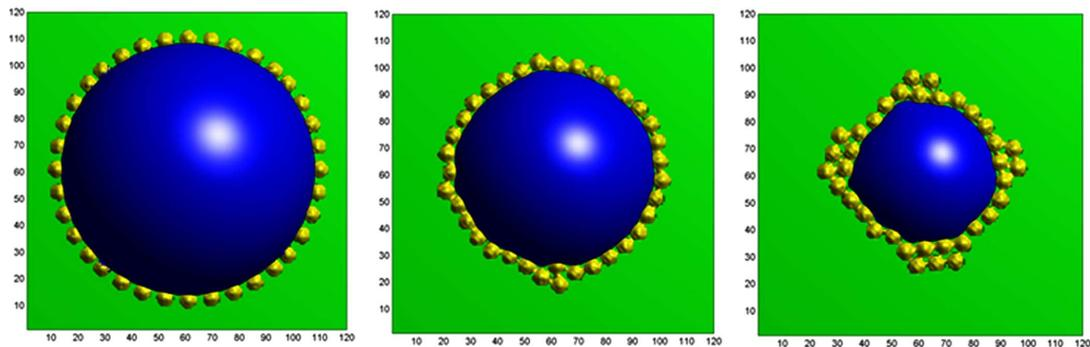
Fig. 10. Shrinking of a 3D liquid drop with particles at the contact line illustrates the tendency of particles to cause jamming of the interface. Particles are eventually ejected from the jammed structure and the drop continues shrinking. The particles eventually form a hexagonal close-packed structure.
