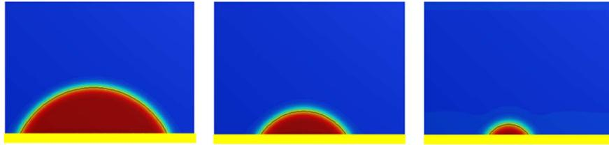
Fig. 6. Simulation of shrinkage (pseudo-evaporation) of a liquid drop using the lattice Boltzmann method. Mass is removed slowly (0.1% at a time) and the system (liquid + vapor) is allowed to return to equilibrium. The contact angle does not change as the drop shrinks.
