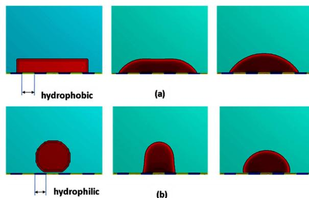
Fig. 5. LBM simulation of contact angle hysteresis (a) An initially rectangular liquid phase relaxing to equilibrium (receding contact angle) (b) An initially circular liquid phase of the same volume relaxing to equilibrium. (advancing contact angle). The final equilibrium shape shows markedly different contact angles.
