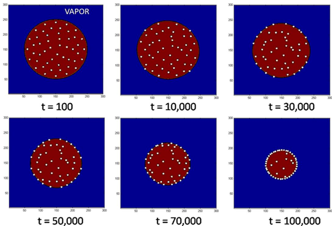
Fig. 9. Shrinking of a free standing, 2D liquid drop containing particles illustrates the tendency of particles to adhere to the shrinking liquid-vapor interface and cause jamming of the interface. A similar jamming effect might help explain contact line pinning with reference to a 3D drop evaporating on a substrate.
