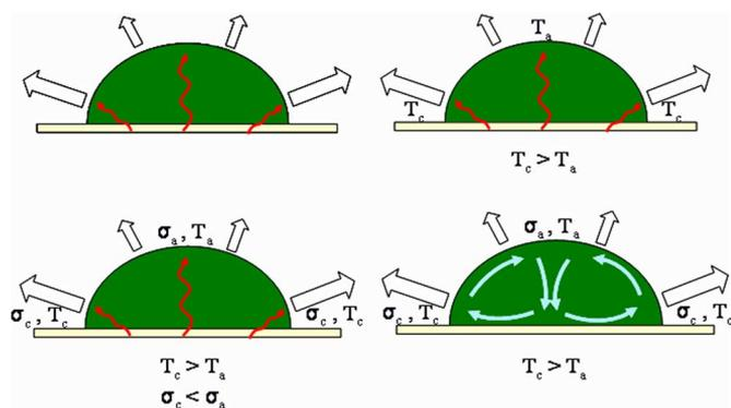
Fig. 2. Schematic depicting the Marangoni flow induced by temperature gradient in an evaporating drop.
