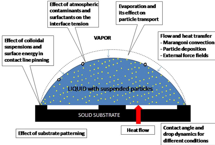
Fig. 3. Physical processes occurring as a liquid drop containing suspended particles impacts on and spreads on a patterned substrate. This work examines the effect of suspended particles on contact line motion and is a first step towards a fundamental understanding of this challenging problem.
