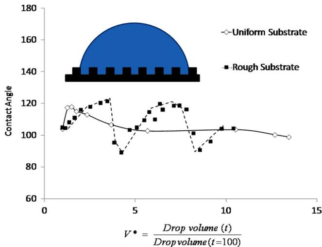
Fig. 7. LBM simulation of a liquid drop shrinking on a rough substrate. The inset illustrates the square-wave profile of the rough substrate and the initial shape of the liquid drop. The graph depicts the stick and slip behavior of the contact angle as the drop shrinks. Because the volume is reducing with time, the initial contact angle corresponds to the maximum  $V^*$  and contact angle evolution with time proceeds from high  $V^*$  to low  $V^*$  (or from right to left on the graph).
