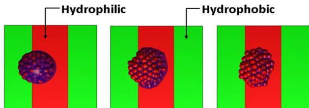
Fig. 11. Colloidal drop dynamics on a patterned substrate comprising of alternating hydrophilic and hydrophobic bands. The drop is initially at rest and contains 87 suspended particles throughout the liquid phase. The snapshots from left to right show the preferential wetting induced by surface energy steps on the substrate and the evaporating process.
