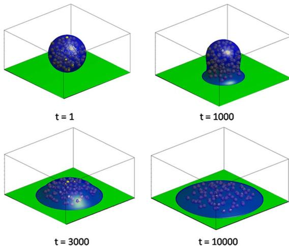
Fig. 8. LBM simulation of a liquid drop containing 90 suspended particles wetting a flat substrate. The particles close to the liquid-vapor interface attach to the interface and the drop eventually attains its equilibrium contact angle of  $30^\circ$ .
