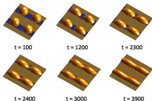
Fig. 4. LBM simulation of drop dynamics on a patterned substrate. The initial shape of the drop is hemispherical and the initial position of the drop is on the hydrophilic (blue) band. Subsequent evolution causes the drop to spread along the hydrophilic band and coalesce with adjacent drops forming a fiber shape. Time is given in lattice units [27].
