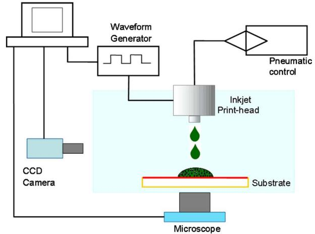
Fig. 1 The ink jet setup
