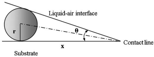
Fig. 5 Schematic representation of the wedge shaped edge of the deposited drop
