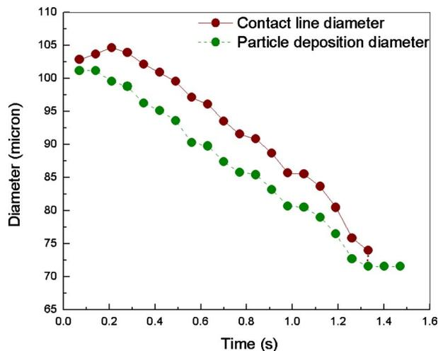
**Fig. 4** The change in contact line and particle deposition diameters with the evaporation of a drop containing  $1.1 \mu\text{m}$  particle suspensions on clean glass substrates
