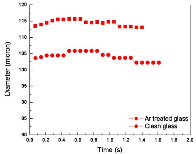
Fig. 12 The variation in contact line diameter with the evaporation of a deposited droplet containing 0.2  $\mu\text{m}$  particles on Ar plasma treated and clean glass substrates
