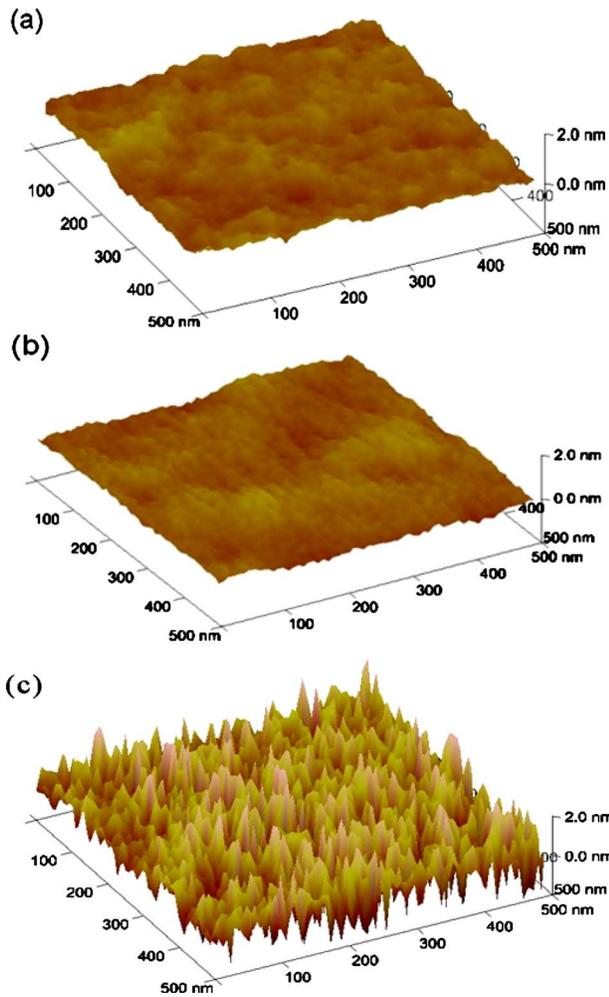
Fig. 11 AFM images of (a) clean glass, (b) Ar plasma treated, and (c) PDMS coated glass samples
