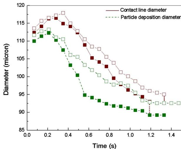
**Fig. 3** The change in contact line and particle deposition diameters with the evaporation of two similar drops, containing  $1.1 \mu\text{m}$  particles on an Ar plasma treated glass substrate (filled squares: drop 1 and hollow squares: drop 2)
