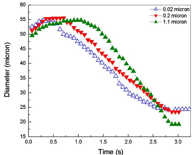
Fig. 8 The variation in contact line diameter with the evaporation of deposited droplets of the three different colloidal suspensions on PDMS coated glass substrates
