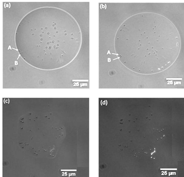
**Fig. 2** Sequence of frames recorded after the impact of a jetted drop containing  $1.1 \mu\text{m}$  particles on an Ar plasma treated glass substrate, (a) just after the impact,  $t=0 \text{ s}$ , (b)  $t=0.28 \text{ s}$ , when the contact line diameter reaches its maxima (c)  $t=0.70 \text{ s}$ , and (d)  $t=1.20 \text{ s}$ , when the drop is completely dried. The pre-impact in-flight diameter and velocity of the drop were  $50 \mu\text{m}$  and  $1.2 \text{ m/s}$ .
