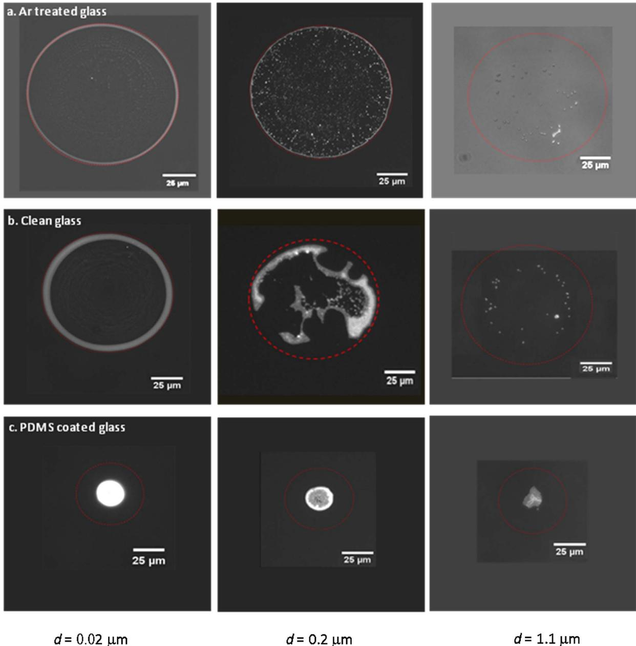
Fig. 10 Microscopic images of inkjet deposited dried droplets of aqueous suspensions of polystyrene particles on (a) Ar treated glass, (b) clean glass, and (c) PDMS coated glass substrates. Each row, from left to right, shows a particle size of  $0.02 \mu\text{m}$ ,  $0.2 \mu\text{m}$ , and  $1.1 \mu\text{m}$ , respectively. The red dashed circles show the maximum diameter position of the contact line with the substrate.
